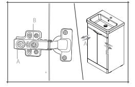
Two door units can be adjusted by the screws on the door hinges.
